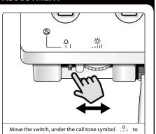
Move the switch, under the call tone symbol . it to adjust the call tone volume level. Move to the centre for a low call tone level and to the right for a high call tone level.
