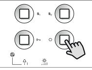
Pick up the handset and then push the camera recall button on as many times as the ID value of the door panel (e.g., if recalling the picture from door ID 2, press this button twice, for door ID 3 press this button 3 times etc.). The videophone display will show the picture from the camera on the relevant outdoor station recalled.
