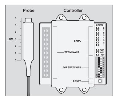
The MD102C is a control unit which enables configuration and testing of the MD102. DIP switches are used for configuration and LED's are used for visual indications of the operation of the probe. A relay output switches ON when a vehicle is detected.
