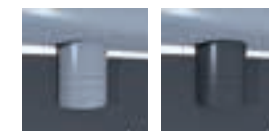
Studs painted the same colour as the frame or the filled section
