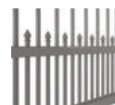
Spacing reduced by adding additional bars and spikes to the base
