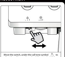
Move the switch, under the call tone symbol  $\stackrel{\triangle}{\hookrightarrow}_{1}$  to adjust the call tone volume level. Move to the left for a low call tone level, to the centre for a medium call tone level and to the right for a high call tone level.
