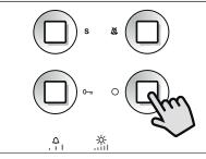
Pick up the handset and then push the camera recall button as many times as the ID value of the door panel (e.g. if recalling the picture from door ID 2, press this button twice, for door ID 3 press this button 3 times etc.).
