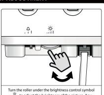
to adjust the brightness of the picture. Any adjustment to the left will reduce the brightness and any adjustment to the right will increase the brightness.
