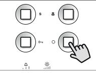
Pick up the handset and then push the camera recall button  $\bigcirc$  as many times as the ID value of the door panel (e.g. if recalling the picture from door ID 2, press this button twice, for door ID 3 press this button 3 times etc.). The videophone display will show the picture from the camera on the relevant outdoor station recalled.
