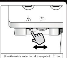
Move the switch, under the call tone symbol  $\begin{bmatrix} \Omega \\ -1 \end{bmatrix}$  to adjust the call tone volume level. Move to the left for a low call tone level, to the centre for a medium call tone level and to the right for a high call tone level.
