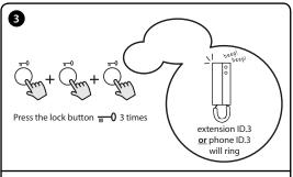
i.e. if calling extension ID.3 or phone ID.3, press the lock button  $0-\pi$  3 times.
