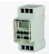
**TH857** is a 7-day, 24 hour digital timer with 6 programmable on/off times each day. Operating at 230Vac, this unit is ideal for providing "free-access" for doors which are electronically locked. The changeover contact is capable of 16Amp switching. An internal battery will store programmed times for up to 200 hours.
